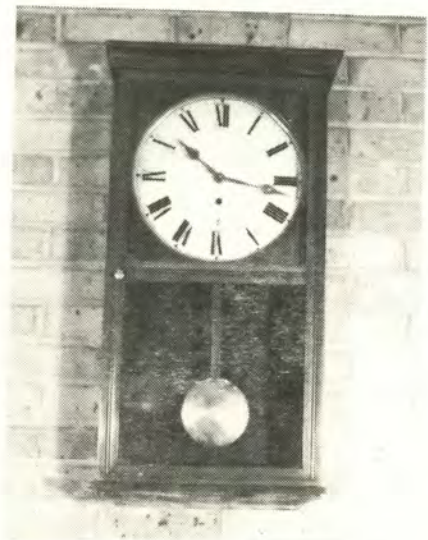
REGULATOR CLOCK, c. 1925 8-Day Time Spring Driven Ansonia Clock Co., Brooklyn, N. Y.
