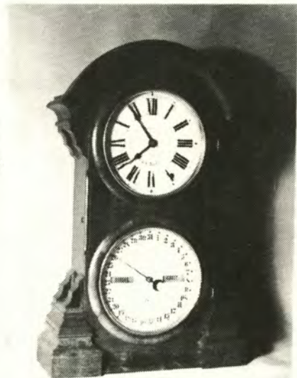
COLUMN CLOCK, c. 1865 30-Hour Time & Strike Weight Driven, Visible Escapement Seth Thomas, Plymouth Hollow, Conn.
