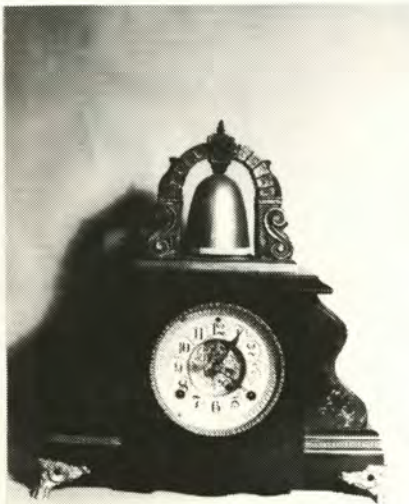
IRON FRONT CLOCK, 1850s 8-Day Time & Strike-Alarm Spring Driven Maker Unknown
