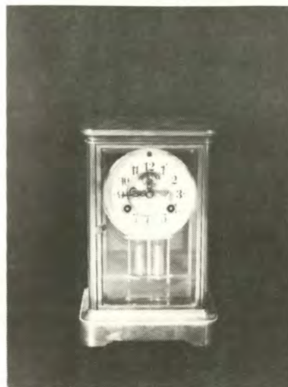
"MORLAIX" CRYSTAL REGULATOR CLOCK, 1900 8-Day Time & Strike Spring Driven; Brocot Escapement Waterbury Clock Co., Waterbury, Conn.
