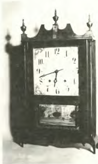
PILLAR AND SCROLL CLOCK, c. 1825 30-Hour Time & Strike Weight Driven Wood Movement E. Terry & Sons, Plymouth, Conn.
