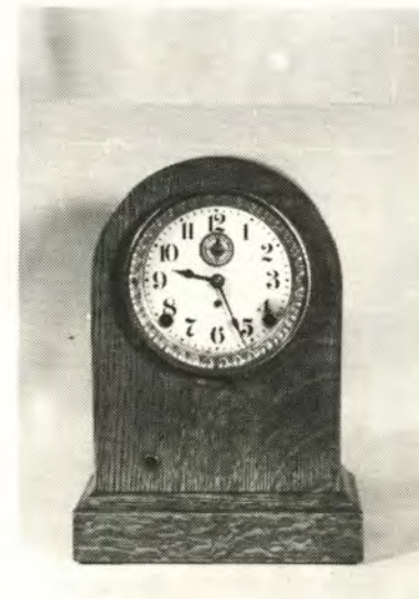
ALARM CLOCK, c. 1885 8-Day Time-Strike -Alarm Spring Driven Seth Thomas Clock Co., Thomaston, Conn.
